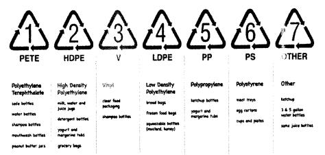
**Note:** PET – Polyethylene terephthalate, HDPE – High density polyethylene, V – Vinyl (PVC), LDPE – Low density polyethylene, PP – Polypropylene, PS – Polystyrene and Other means all other resins and multi – materials like ABS (Acrylonitrile butadiene styrene), PPO (Polyphenylene oxide), PC (Polycabonate), PBT (Polybutylene terephalate) etc.
